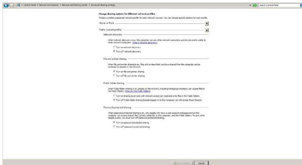
Figure 15 Network and Sharing Center >> Change Advanced Sharing Settings >> Turn on File and Printer Sharing
